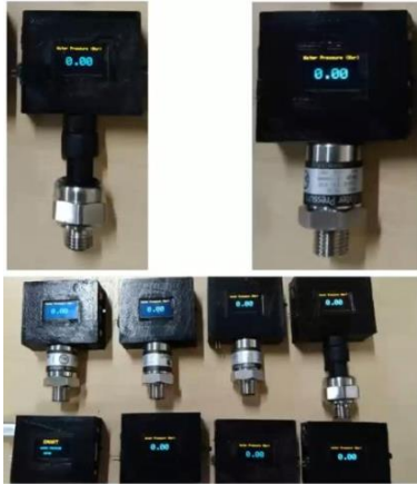
Pressure Sensors – Ambuj Range: 0 – 5 bar and 0-50 bar
