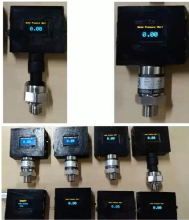
Pressure Sensors – Ambuj Range: 0 – 5 bar and 0-50 bar
