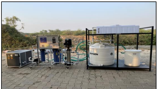
Lab skid NF/RO performance testing unit to test the performance of the NF and RO membrane
